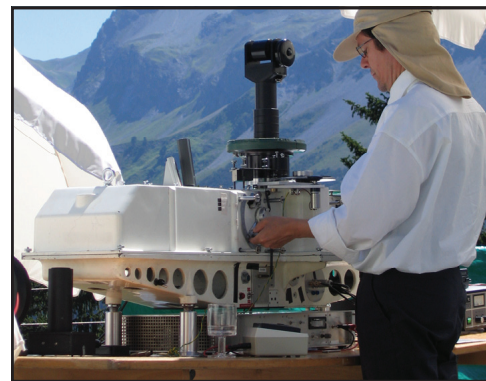
Figure 29. Data from ground-based instruments, like this Dobson spectrophotometer in Arosa, Switzerland, didn't seem to show any decrease in ozone levels. What was going on?
