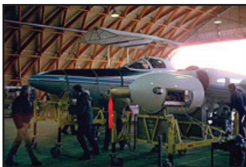
Figure 27. The specially equipped NASA research aircraft that gathered much of the data used in James Anderson's study of the Antarctic ozone hole. The wing pod in the center foreground contains the instrument for measuring chlorine monoxide concentrations in the upper atmosphere.
